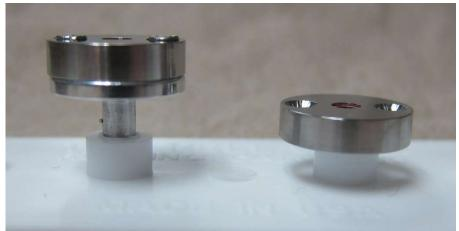
Two views of the MRS-6 retainer (SS304) are shown above. The top section holds the MRS-6 and is 12.5 mm X 3 mm. The bottom is a 3 mm aluminum pin. The MRS-6 is approx. 0.2 mm below the top surface secured by a "C" clip from below.
